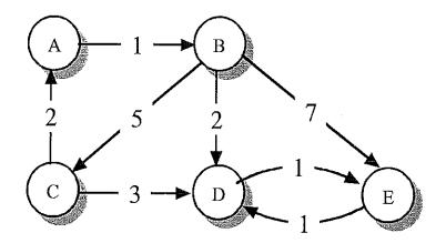
A graph is represented by G = (V, E), where V is the set of vertices (or nodes), E is the set of edges of the graph. The above graph represents locations of warehouses of a company with the distance between them.
