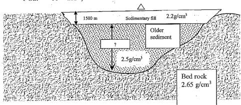
$g = 2\pi G\rho z$ ; Gravity effect of horizontal cylinder = uniform density =  $\rho$ ;
