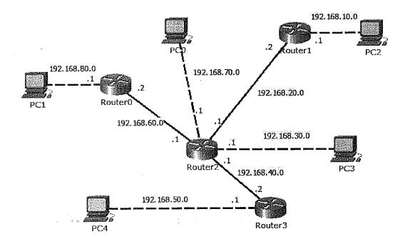
a) Write the commands that are required in configuring each router (Router 0 to Router 3) for static routing in the given topology.
