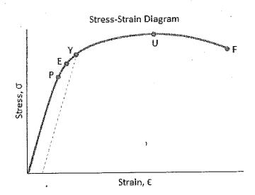
(iii)Referring to the structure and behavior of the metal under a tensile force, explain about the each point P, E, Y, U, and F. (5 Marks)
