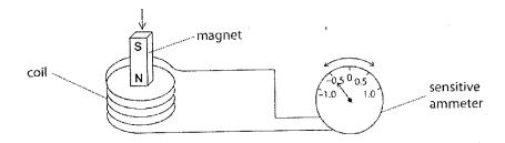
The moving magnet and the coil of wire are producing an electric current. The magnitude and direction of the current can be changed in a number of ways. **Describe** changes that can be made to produce different currents and the effect of each change. (05 Marks)
