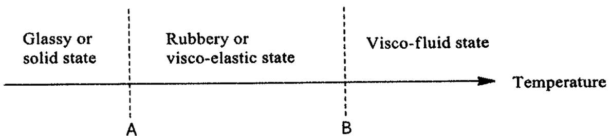
(vi) The changes of thermal expansion coefficient value of a particular polymer sample at different temperatures have been shown in the following figure with respect to a particular study.
