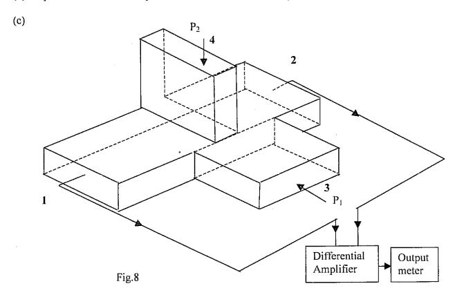
Fig. 8 shows a microwave phase detector circuit using a Magic Tee. The two signals (signal powers  $P_1$  and  $P_2$ ), equal in magnitude but different in phase are fed at ports 3 and 4 respectively.
