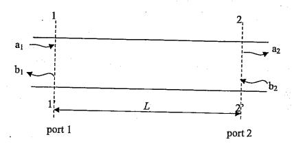
Incident- and the reflected waves are represented by  $a_n$  and  $b_n$  respectively (n = 1, 2; m = 1, 2). Assuming that the line is lossless and the phase constant to be  $\beta$ , write the relationship between
