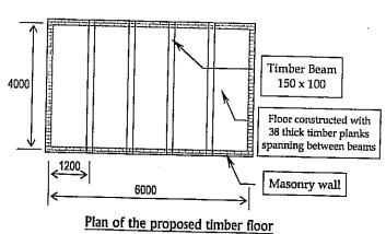
The floor layout consists of timber planks supported by timber beams which are simply supported on existing masonry walls as shown .Effective span of a timber beam is 4.0 m and they are spaced at 1.2 m.
