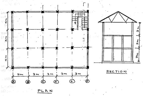
There is a 200 mm thick masonry wall along the perimeter. All internal partitioning is done using light weight materials.
