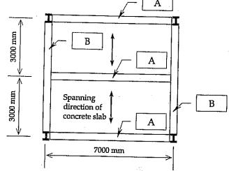
Design the universal steel beam 'A', using grade S275 steel, assuming that the top flanges are fully restrained by the concrete slab. In the process consider the most critically loaded beam and follow following steps;
