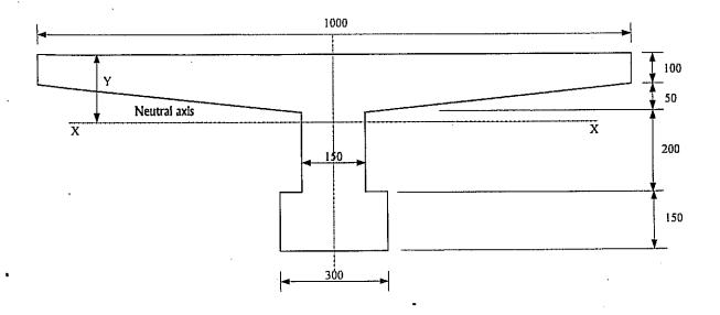
Based on preliminary calculations the Design Engineer has selected the above cross section and the following, material properties and probable loading on the floor applicable to the proposed prestressed beam;
