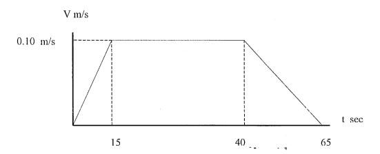
The motor first accelerates for a period of 15 s and attains a speed 0.10 m/s, which is uniformly maintained for the next 25 secs. Finally the motor is switched off, so that the load reaches the unloading bay at the 65<sup>th</sup> second under the application of brakes. Once unloading is complete, the reverse gear is engaged and the motor is
