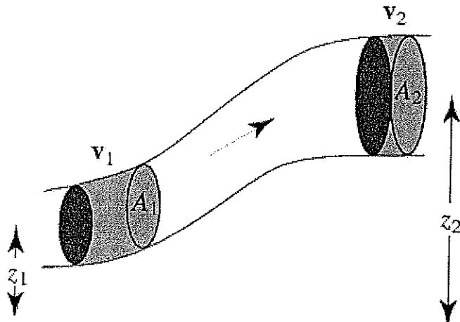
$A_1$ = cross sectional area of the pipe at narrower end
