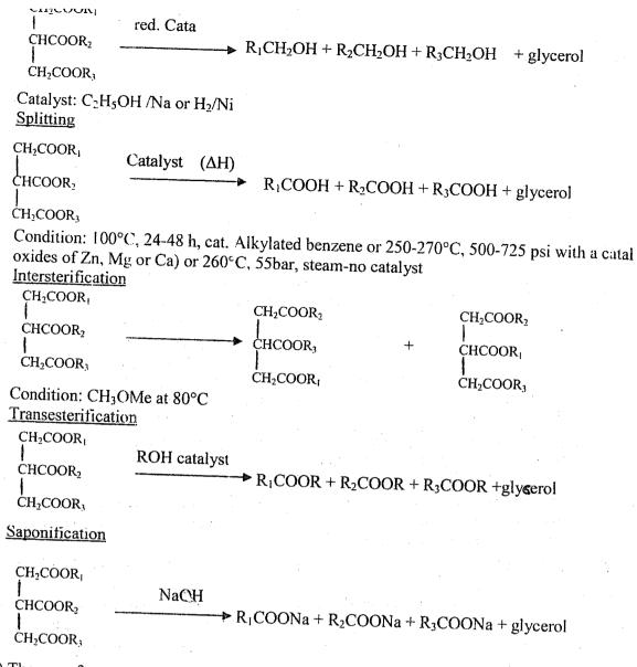
c) There are 3 processes of soap manufacturing. Cold process, semi-boiled process and full-be process. In soap manufacturing latty acids and NaOH or KOH are used as raw materials. Bu detergent manufacturing other than them strong cationic or strong anionic compounds are all used.
