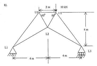
Figure 2 shows a pin-jointed frame, which is hinged to the support at L1 and on a roller support at L3. Take EA as constant for all members.
