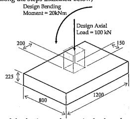
i.) Check for soil bearing and possibility of lifting of the footing, under service loads and propose modifications if necessary,
