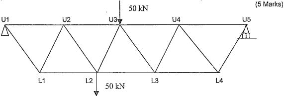
2 A pin-jointed frame is hinged to the support at U1 and on a roller support at L3 as shown in the figure below. Take EA as constant for all members.
