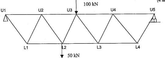
2. a). Describe the method of finding out displacement of C of truss shown below with "Williot displacement diagram method". (7 Marks)
