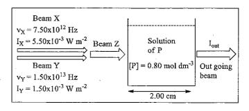
The frequencies of the radiation in beams X and Y were  $7.50\times10^{12}$  Hz and  $1.50\times10^{13}$  Hz, respectively. The intensities of them were  $5.50\times10^{-3}$  W m<sup>-2</sup> and  $1.50\times10^{-3}$  W m<sup>-2</sup>, respectively. Concentration of P was  $0.80 \text{ mol dm}^{-3}$ . The path length of the cell used was 2.00 cm. Molar extinction coefficient of P at radiation frequency  $7.50\times10^{12}$  Hz, is  $0.50 \text{ mol}^{-1} \text{ dm}^3 \text{ cm}^{-1}$ .
