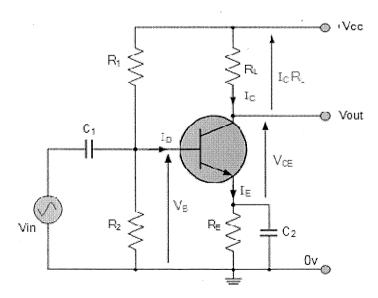
c) Assuming the use of a Silicon based transistor, with  $R_1$  = 27 k $\Omega$ ,  $R_2$  = 14.7 k $\Omega$ ,  $R_E$  = 680  $\Omega$ ,  $R_L$  = 1 k $\Omega$ ,  $V_{CC}$  = 10 V and  $\beta$  = 100, calculate the Currents  $I_B$ ,  $I_C$  and the Voltage  $V_{CE}$ . (8 marks)
