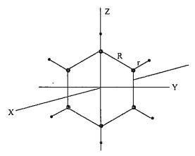
X is perpendicular to the plane of the molecule. Y and Z are in the plane of the molecule. All three axes passes through the centre of mass of the molecule and are mutually perpendicular. Denote the masses of C and H by M and m and C—C and C—H bond lengths by R and r.
