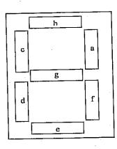
ii. Design a circuit for any three values of BCD-to-7 Segment decoder.
