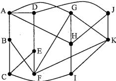
Find a spanning tree of minimum height of the above graph by using the *Breadth First Search* algorithm.
