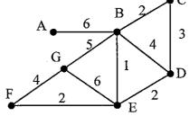
Verify the above result using Prim's Greedy algorithm, by starting with the edge AB.
