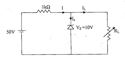
In the above circuit determine the range of  $R_L$  that will result in a constant voltage of 10 V across  $R_L$ .
