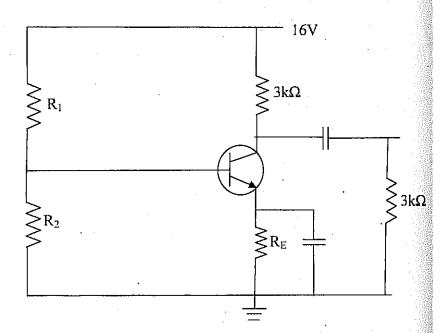
Establish the relation  $\beta=\frac{\alpha}{1-\alpha}$  for a bipolar junction transistor. In the above circuit npn transistor has  $\alpha=0.985$  and  $V_{BE}=0.3V$ . Calculate  $R_1$ ,  $R_2$  and  $R_E$  to place the Q-point at  $I_C=2mA$  and  $V_{CE}=6V$ . Draw the dc and ac load lines of the circuit.
