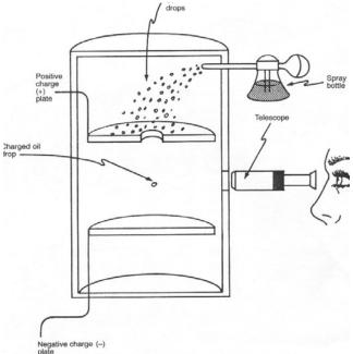
droplet picked up a slight charge of static electricity as it traveled through the air, the speed of its motion could be controlled by altering the voltage on the plates. When the space between the metal plates is ionized (by radiation), electrons from the air attach themselves to oil droplets, causing them to acquire a negative charge.
