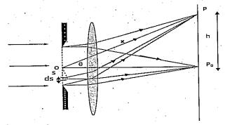
for the displacement  $dy_0 = a (ds/X) Sin (\omega t-kX)$  of the wavelet at P coming from the element ds, situated at the origin. where "a" is the amplitude at ds, X is the distance traversed by the wavelet and  $k = 2\pi/\lambda$  is the wave number and " $\omega$ " is the angular frequency. [60 marks]
