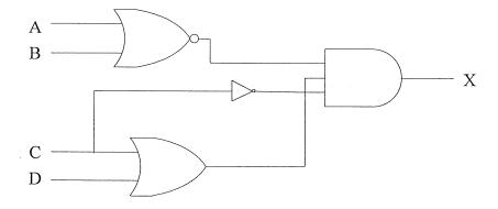
e. **Substitute** all the gates in the simplified circuit in the section (d) above using **NAND** gates and **simplify** the circuit again, if necessary.
