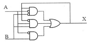
(iv) Identify the race conditions in the asynchronous circuit in Q5 (iii) and mention the steps you take to remove the race condition.
