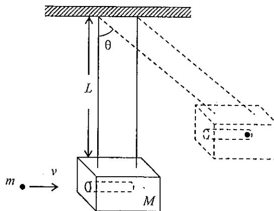
The bullet (of mass  $m$ , in the form of a small metal ball) is ‘fired’ horizontally towards a block of wood (of mass  $M$ , in which a hole has been drilled) suspended from two vertical inextensible strings (each of length  $L$ ). On striking the block, the bullet is embedded and the block rises by swinging through an angle  $\theta$  as shown.
