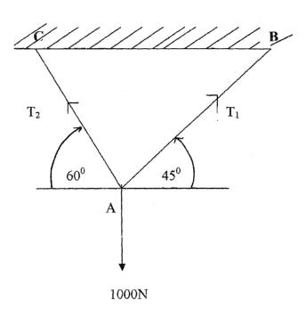
A 1000 N weight object is hanging from A. (see above figure) using two string AB and AC connected to two points B and C in horizontal roof. Find  $T_1$  and  $T_2$  the tension of the two strings AB and AC.
